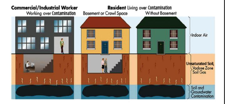
directly within confined spaces (basements, crawl spaces, etc.). The concentration of the vapors are calculated, and if necessary, run through a model to determine the potential exposure to workers and residence based on factors that include the likely length of time that individuals may be exposed on a daily or annual basis. If the calculations or models indicate that a potential health threat exists, the regulatory agency will require abatement of the vapor.
